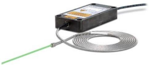
The picosecond pulsed laser diode heads of the LDH-FA Series are based on a Master Oscillator Fiber Amplifier (MOFA) concept with optional frequency conversion.
